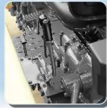
iPTO Clutch Independent hand lever for operating PTO clutch, better clutch life & ease of operations
